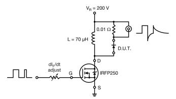
Fig. 10 - Reverse Recovery Parameter Test Circuit
