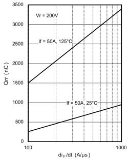
Fig. 7 - Typical Stored Charge vs. dl<sub>F</sub>/dt
