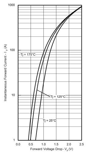
Fig. 1 - Typical Forward Voltage Drop Characteristics (Per Diode)
