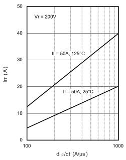
Fig. 9 - Typical Stored Current vs. dl<sub>F</sub>/dt
