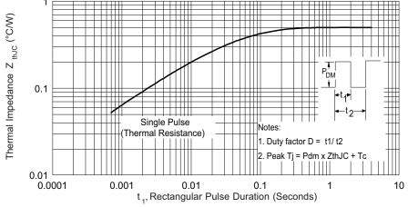
Fig. 3 - Maximum Thermal Impedance Z<sub>thJC</sub> Characteristics (Per Diode)
