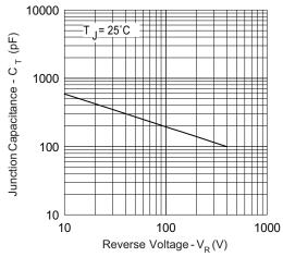
Fig. 2 - Typical Junction Capacitance vs. Reverse Voltage
