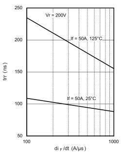
Fig. 6 - Typical Reverse Recovery Time vs.  $dI_{\text{F}}/dt$
