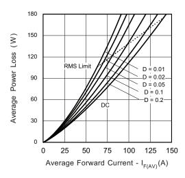
Fig. 5 - Forward Power Loss Characteristics (Per Leg)
